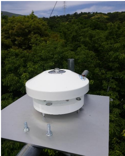
a) Installed View of MS-700 for Downwelling Irradiance Observation
