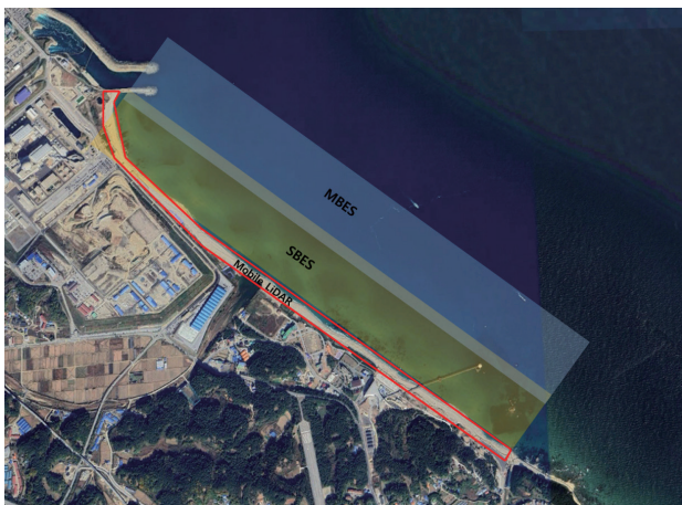
Fig. 1. Survey area. MBES, multi-beam echo sounder; SEBS, single-beam echo sounder.
